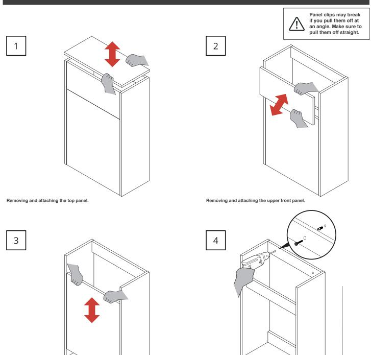
Drill two holes to fix the unit to the wall.
